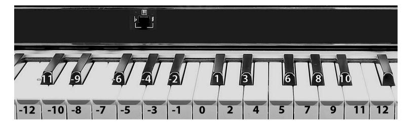
The transpose button is labeled with a small keyboard icon and has a red LED that turns on whenever the transposition is active. **Transposition is always zeroed every time the instrument is turned on.** To change the transposition between -12 and +12 semitones, just press and hold the transpose button and play a note around the middle C. To reset, use the middle C or keep the transpose button depressed for 3 seconds until the LED goes off.
