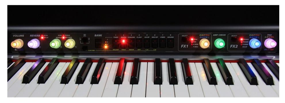
Since most of the knobs don't need to be set to a precise value, a numerical readout is unnecessary (even a potentiometer can't give a precise readout), so the idea is to have the knob change color according to the current value, towards green when the value is low and towards red when the value is high, with intermediate shades of colors in between.
